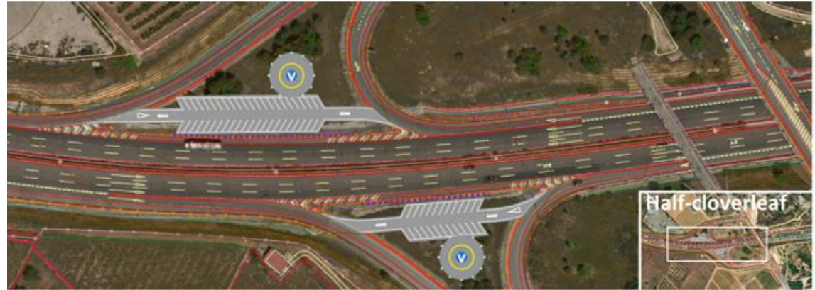
Fig. 13. Safe Harbor located in a half-cloverleaf.
