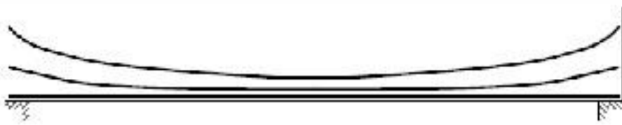
Inclined longitudinal reinforcement
