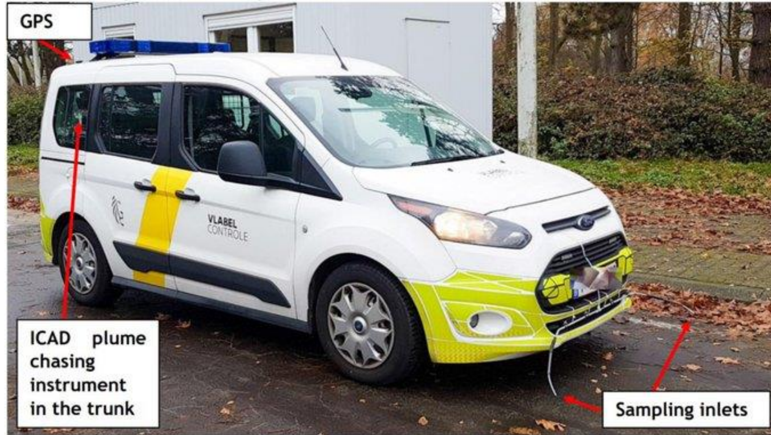
Figure 4: Plume chasing installation on the Vlabel Controle vehicle (outside view). Two sampling inlets are combined to one sampling hose to the ICAD plume chasing instrument in the trunk.
